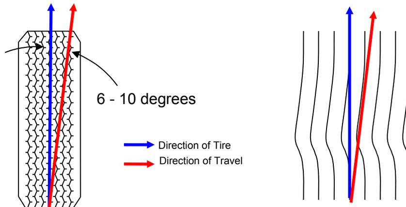
So the tire producing a "Slip Angle" isn't really slipping across the pavement, it's merely being tweaked so much that it actually begins steering itself to the outside of the turn. In poor grip conditions, such as rain and snow, our slip angles are in fact caused by the tire literally slipping across the surface of the road, but in doing so they may not necessarily be generating the greatest possible grip (which is another subject entirely).
